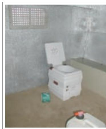
*Chemical toilet provided within the compartment of Isuzu vans. Both the toilet and water container are unanchored.*
