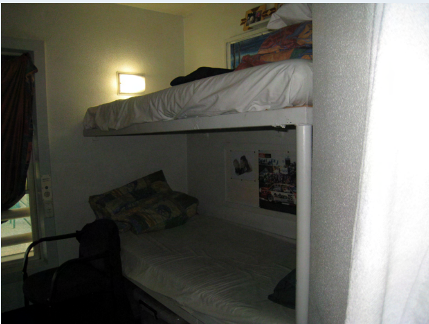
'Old' design bunks in the self-care unit. Prisoners climb on the chair to get in. Note that there are no guard rails to prevent 'roll out'.
