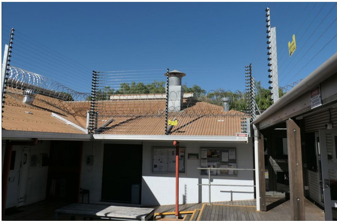
Photo 17: The pulse energised fence improved security in the female unit but was imposing.
